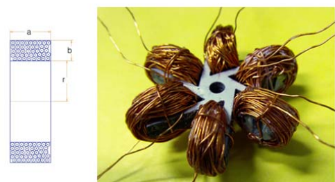
Figure 4. Left – dimension of short cross-wound coil. Right – real winding of coil
